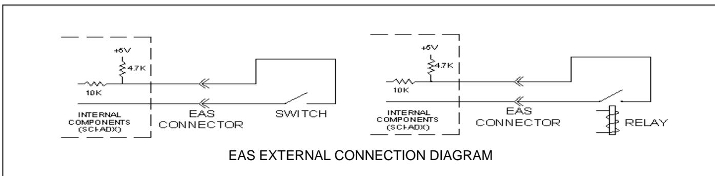
When the EAS is activated, all serial (RS-232 & RS-422) input to the SCI-ADX is ignored. Also, any pending commands in the serial buffer are flushed.
