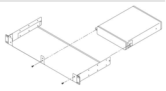
2) FASTEN UNIT TO FRAME WITH TWO SCREWS.
