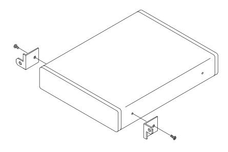
\* NOTE: FOUR (4) MOUNTING BRACKETS AND EIGHT (8) #6-32 SCREWS ARE SHIPPED WITH THE RMT-2100-2.
